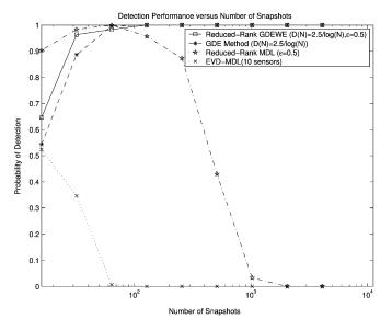
Fig. 8. Probability of correct detection versus number of snapshots in the case of spatially inhomogeneous noise.  $[\theta_1, \theta_2] = [0.5^\circ, 6.2^\circ]$ , SNR = 5 dB, WNPR = 10, L = 10, and N varies from 16 to 4096.
