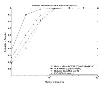
Fig. 6. Probability of correct detection versus number of snapshots for the case of spatially white noise.  $[\theta_1, \theta_2] = [0.5^\circ, 6.2^\circ]$ , SNR = 0 dB, L = 10, and N varies from 16 to 1024.
