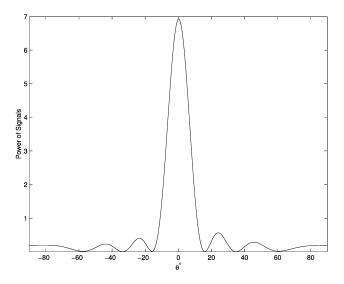
Fig. 1. Response of the spatial matched filter  $r_{x_0d_0}$ . The direction of a single incident signal is 0°, the number of sensors is 8, and SNR equals 0 dB.
