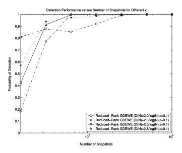
Fig. 5. Probability of correct detection of the GDEWE versus number of snapshots for different  $\kappa$  in the case of spatially white noise.  $[\theta_1, \theta_2] = [0.5^\circ, 6.2^\circ]$ , SNR = 0 dB, L = 10, and N varies from 16 to 1024.
