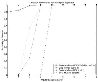
Fig. 7. Probability of correct detection versus angular separation  $(\Delta \theta)$  for the case of spatially white noise.  $[\theta_1, \theta_2] = [0.5^{\circ}, \theta_1 + \Delta \theta]$ , SNR = 5 dB, N = 256, L = 10, and the angular separation varies from 0° to 0°.
