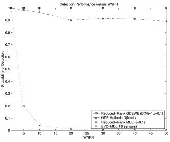
Fig. 10. Probability of correct detection versus WNPR.  $[\theta_1, \theta_2] = [0.5^\circ, 6.2^\circ]$ , SNR = 5 dB, N = 256, L = 10, and WNPR varies from 1 to 50.
