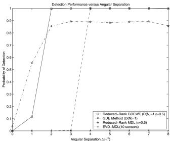
Fig. 9. Probability of correct detection versus angular separation in the case of spatially inhomogeneous noise.  $[\theta_1, \theta_2] = [0.5^\circ, \theta_1 + \Delta\theta]$ , SNR = 10 dB, N = 256, WNPR = 10, L = 10, and  $\Delta\theta$  varies from 0° to 8°.
